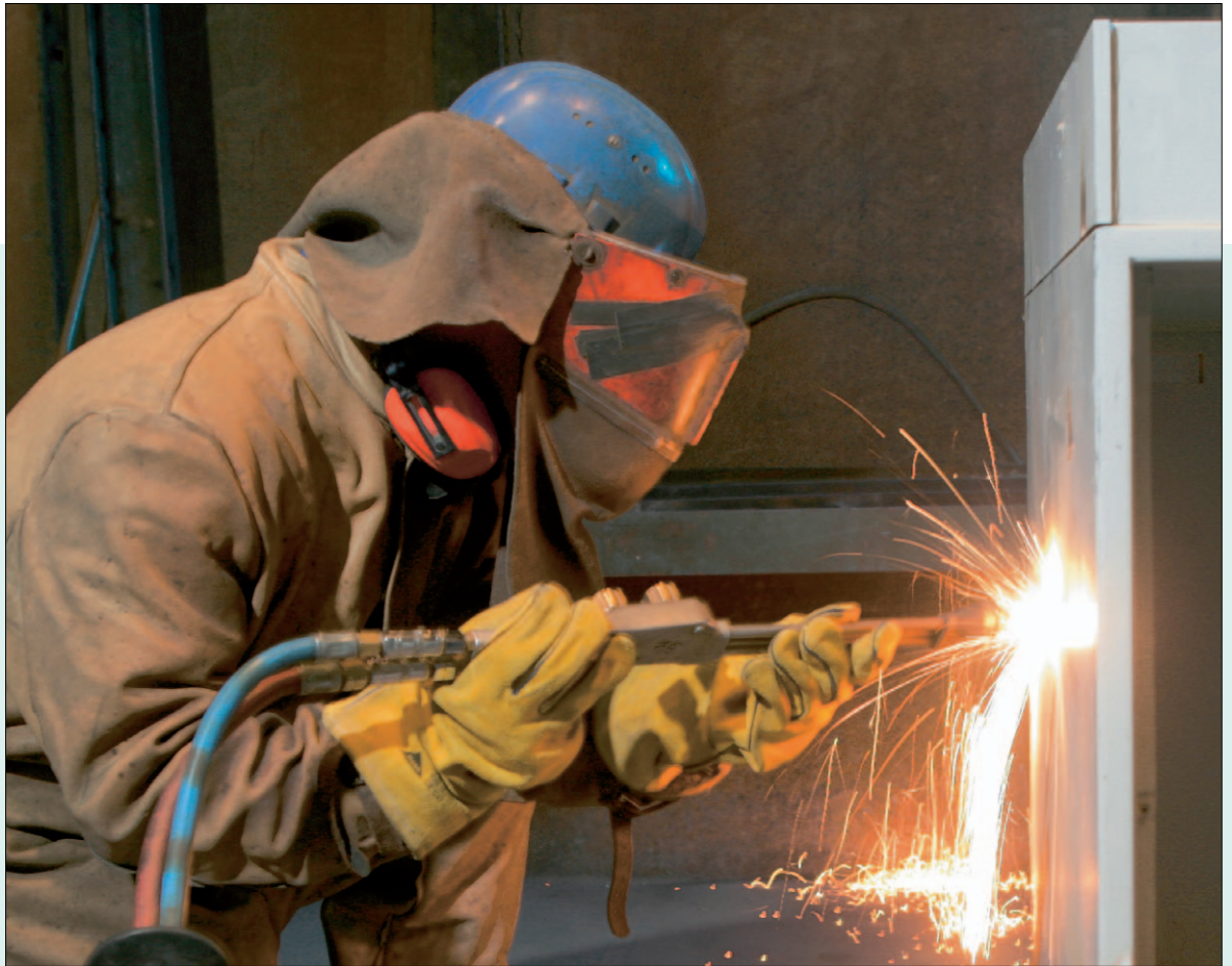
Thermal attack on a safe at VdS laboratories
